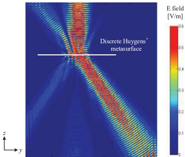
Fig. 4. The electric field magnitude distribution of the designed metasurface upon normally incident Gaussian beam.
