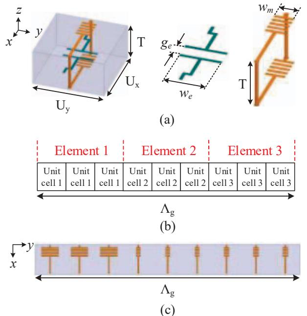
Fig. 3. (a) Geometric structure of a unit cell. The three metallic layers consisting electric and magnetic dipoles are all perfect conduct. (b) A schematic diagram of a period of the metasurface. (c) Top view of a period of the designed metasurface, with only the top metallic layer visible.
