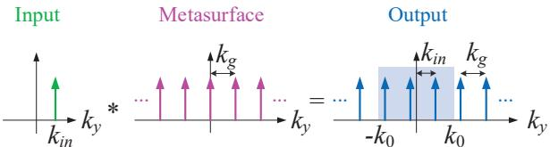
Fig. 1.  $k$ -space operation of a periodic metasurface which varies along  $y$ -direction. Arrows indicate the existence of an infinite number of diffraction modes, the light blue box denotes the free space propagation range from  $-k_0$  to  $k_0$ .
